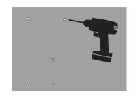
For wall-mount, fix the backplate using 5 PA6\*50mm tapping screws. For pole-mount, fix the backplate using 5 M5\*16mm
